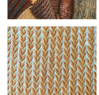
SHILEAD introduces WTS-XLD206A, which contains 23% Circulose, developed by the Swedish Company Re:newcell. The production process uses the waste textile to make pulp and spins it into visose fiber. This yarn is blent with linen and recycle polyes-
